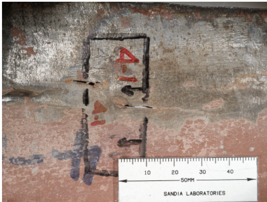
Figure 53. Details of inside (top) and outside (bottom) liner features in region of tear #4-1 metallographic cross-section (arrows begin at plane of section and indicate view direction).
