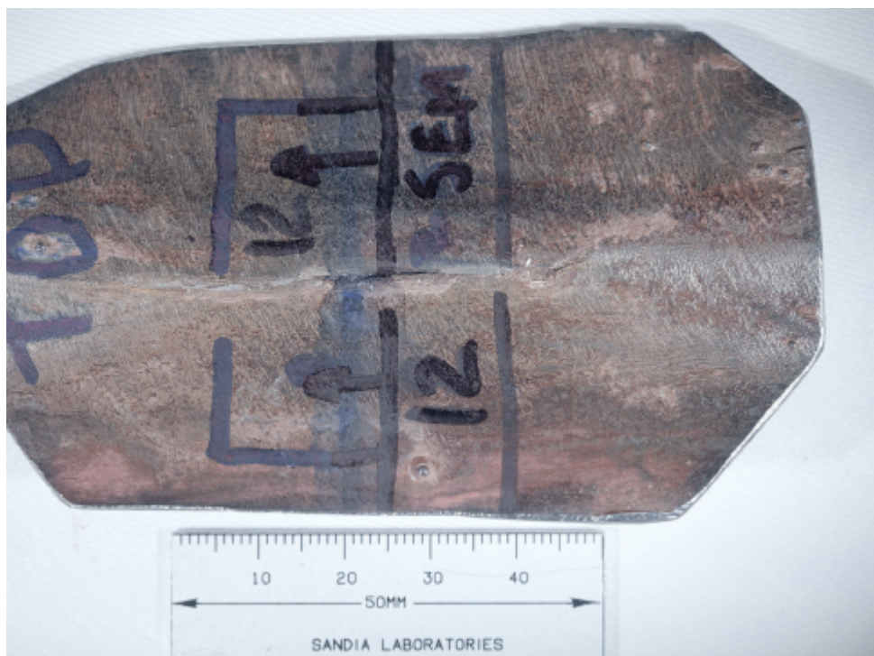
Figure 62. Details of inside (top) and outside (bottom) liner features in region of tear #12 metallographic cross-section (arrows begin at plane of section and indicate view direction). Location of SEM fractographic sample is also shown.
