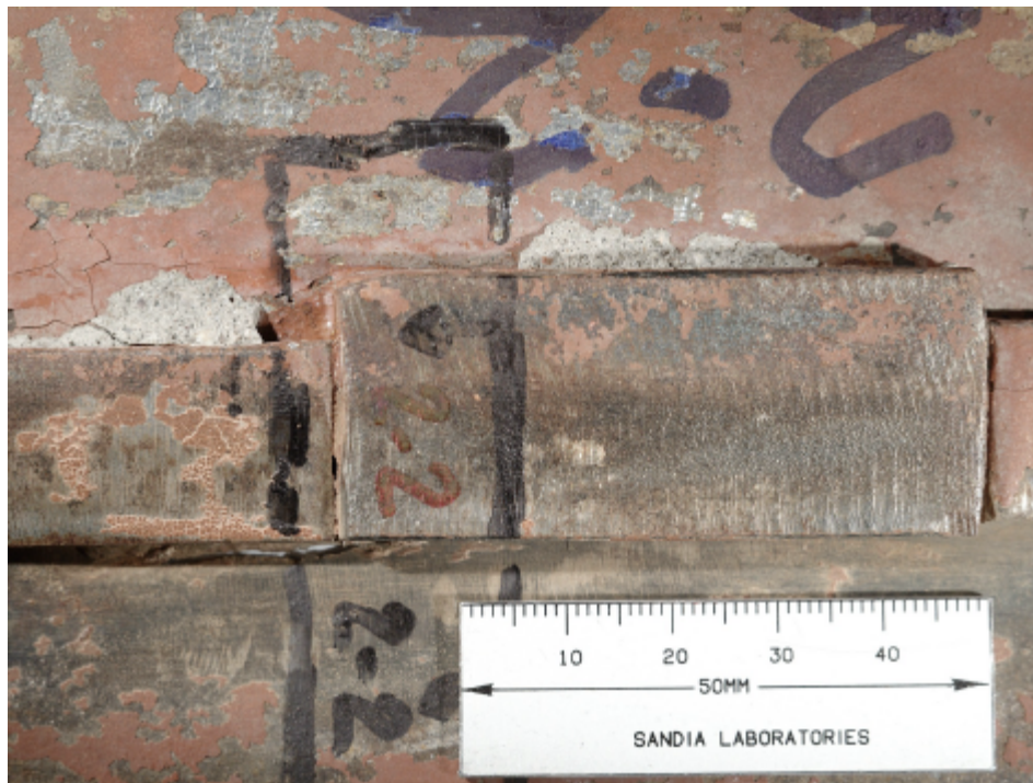
Figure 51. Details of inside (top) and outside (bottom) liner features in region of tear #2-2 metallographic cross-section (arrows begin at plane of section and indicate view direction).
