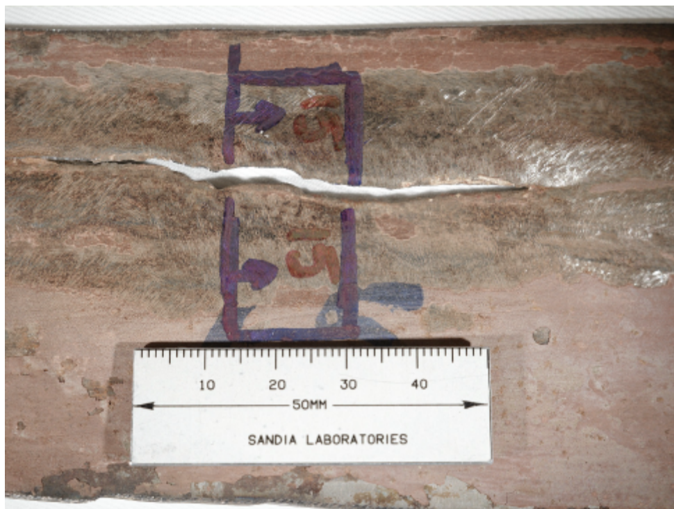
Figure 61. Details of inside (top) and outside (bottom) liner features in region of tear #15 metallographic cross-section (arrows begin at plane of section and indicate view direction).
