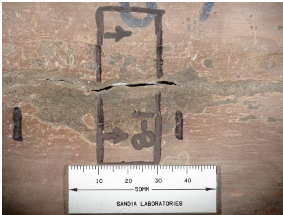
Figure 56. Details of inside (top) and outside (bottom) liner features in region of tear #8-1 metallographic cross-section (arrows begin at plane of section and indicate view direction).
