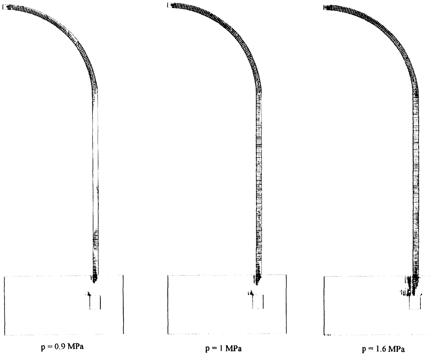
Fig. 19. Meridional cracking pattern for various pressure levels
