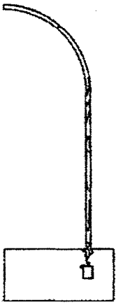
(iv) cracking at pressure 1240 kPa
