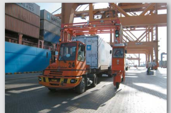
The Megaports Initiative's Mobile Radiation Detection and Inspection System offers a versatile and flexible solution for radiation detection of shipping containers in a port environment.
