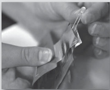
A hands-on demonstration of a 20 mA Li-ion battery bent around a 1.8 V red LED.
