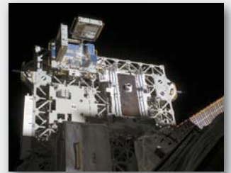
MISSE-7 suitcase-like containers hold Sandia experiments on the exterior of the International Space Station. White rectangular box is SEUXSE; orange boxes contain passive Sandia-developed advanced materials and components.
