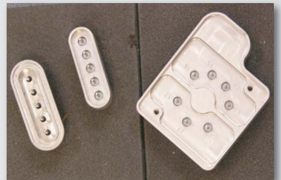
W76-1 Intent Stronglink headers with a novel glass-ceramic materials system that improves performance and manufacturability while also significantly reducing cost.
