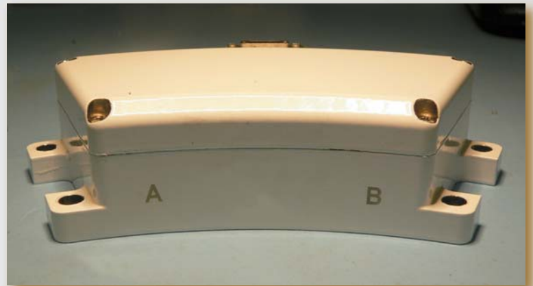
Neutron generator monitor.
