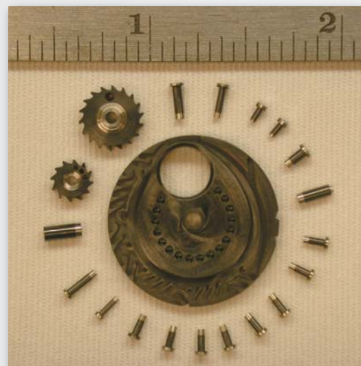
Diamond-like nanocomposite (DLN)-coated dual stronglink mechanism parts.
