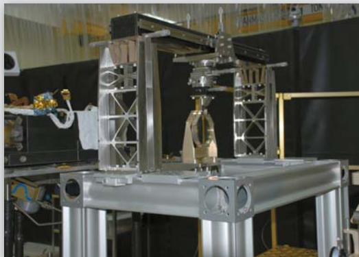
Gantry system, conceived and designed by Dept. 2617 staff, used to align a lens cell assembly for optical testing. The system allowed alignment tolerances in the ten-thousandths range to be maintained to meet system performance requirements.
