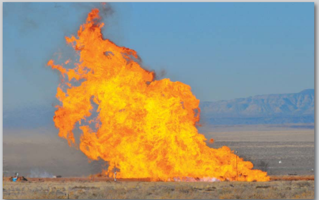
LNG fire on water, 23-meter diameter. (Photo by Randy Montoya)
