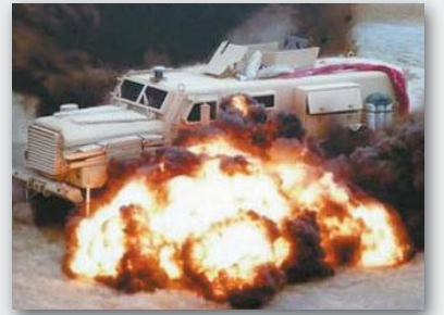
Mine Resistant Ambush Protected Vehicle undergoing testing.
