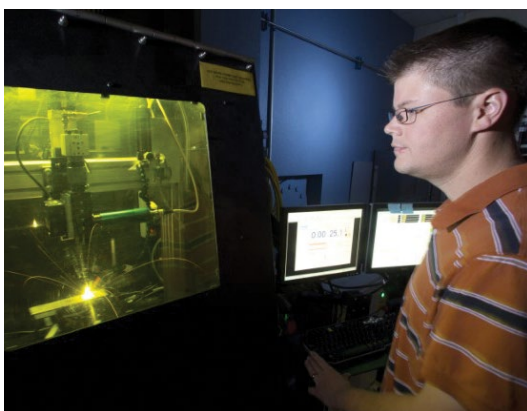
Cody Love laser welds an explosive component.
