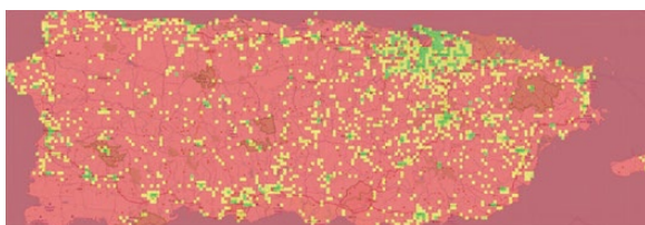
Sandia's Resilient Node Cluster Analysis Tool identifies locations in Puerto Rico for resilient microgrids that provide the best (green) or good (yellow) access to services, based on a variety of social and infrastructure parameters.
