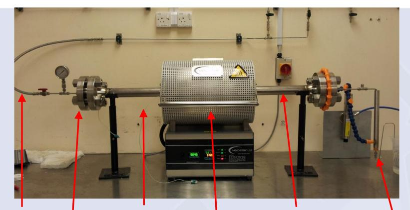
Gas supply Thermocouple wire Alloy 625 vessel body Sealing flange Split-tube furnace Cooled gas vent
