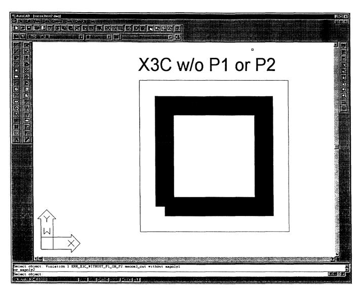
Figure 6. DRC Result Example - Missing Geometry
