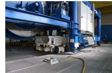
Emplacement machine towing with the transport cart and the locomotive
