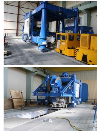
Emplacement machine towing with the transport cart and the locomotive
