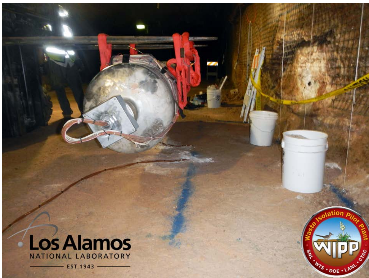
Figure 48: End view of canister. Salt pile will connect from canister to wall; pile-wall interface is an area of interest. Blue markings on floor indicate measurement lines for canister placement.
