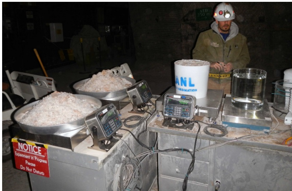
Figure 41: Salt pan experiment in WIPP salt gallery. Pans with salt piles are on left.
