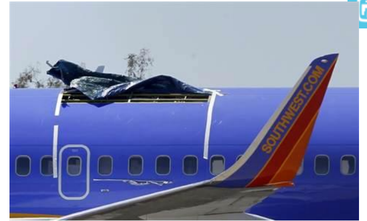
Roof failure of Boeing 737 aircraft due to fatigue cracks. From imechanica.org
