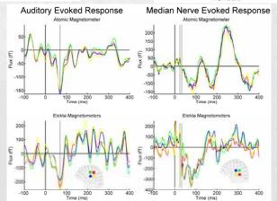
Replication of left hemisphere response to auditory stimulation with 1000 Hz tones comparing the atomic magnetometer and Elekta
