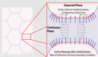
Viscosity at an interface can be vastly different from the continuous phase
