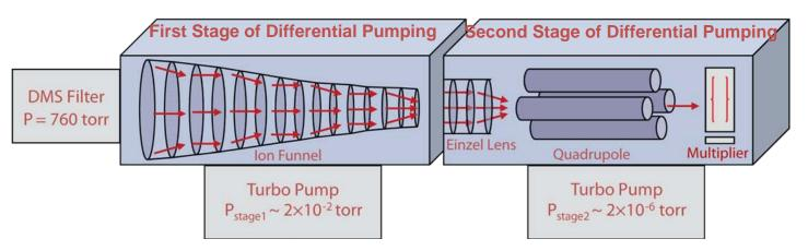
Ion transport modeling used to design 50 lens element RF "ion funnel" for radial confinement
