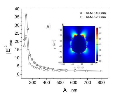
Simulations show an Al-NP (100 nm diameter) increases the electric field by 35 fold at ca. 285 nm (toluene emission frequency).
