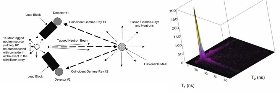
Using the Triple Coincidence Technique to Detect DU
