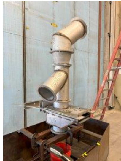
Testing of particle flow within the isolation valve
