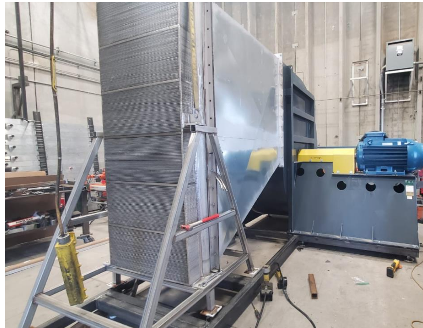
sCO 2 blower (right) and air cooler HX (left)
